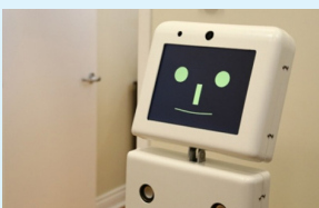
The ED mobile robotic system is voice activated and interacts with the user through audio and video
